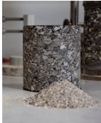
Aggregate recovered from WTE operations that can be used in road and other construction projects
