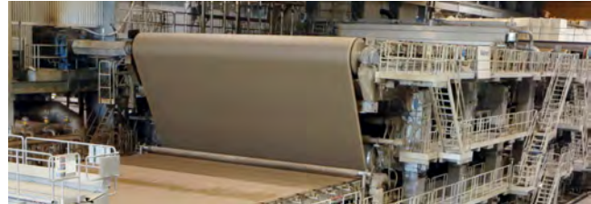
Greenpac Mill uses waste-to-energy steam produced by Covanta Niagara in its process, including for drying the 100% recycled paper.
