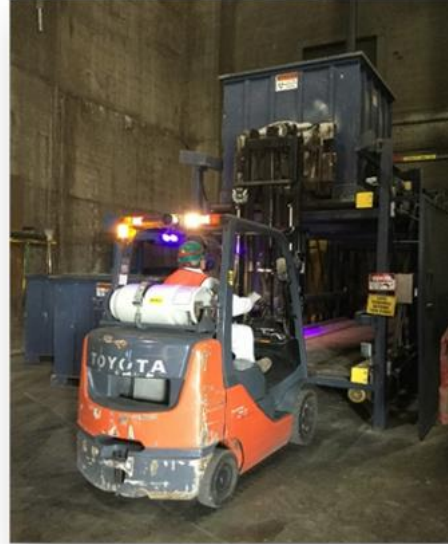
Figure 5 - WFS conveyors at tipping floor grade elevation. Figure 6 - Example of forklift loading the upper Tipping Floor Supply Transfer conveyor.
