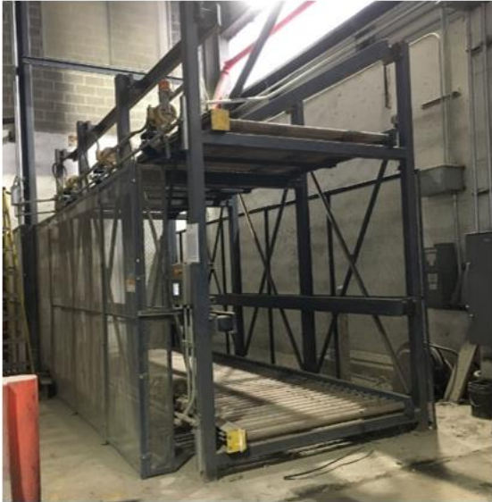
Figure 5 - WFS conveyors at tipping floor grade elevation. Figure 6 - Example of forklift loading the upper Tipping Floor Supply Transfer conveyor.
